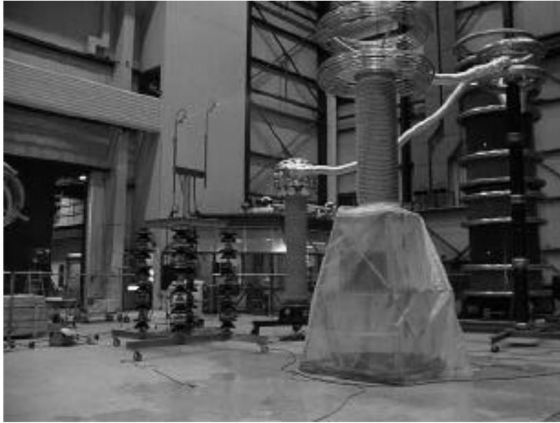
Figure 2. Wet tests on the NXVT.
