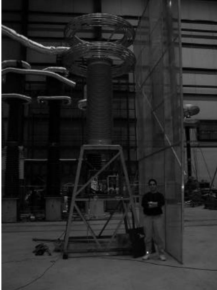
Figure 1. The NXVT together with a ground plane for testing the effects of field distribution changes on the NXVT measurements.
