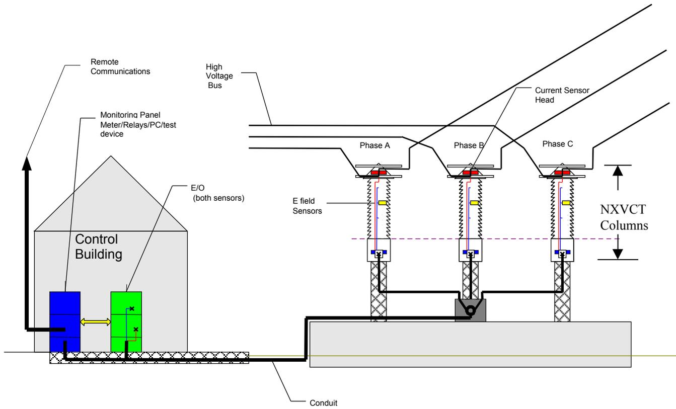
Figure 4. Field Trial Schematic
