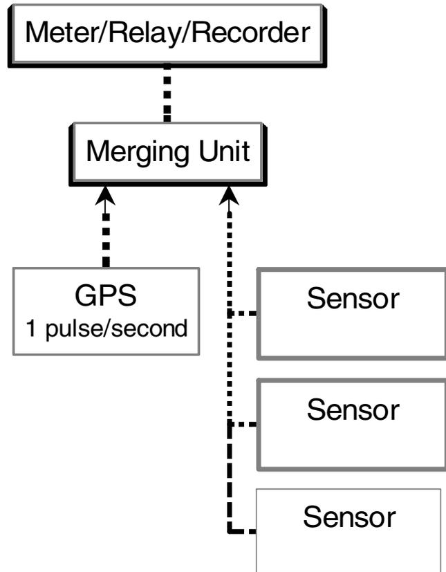
Figure 2. The digital architecture according to IEC 60044-8 and IEC 61850-9-2 is shown above.
