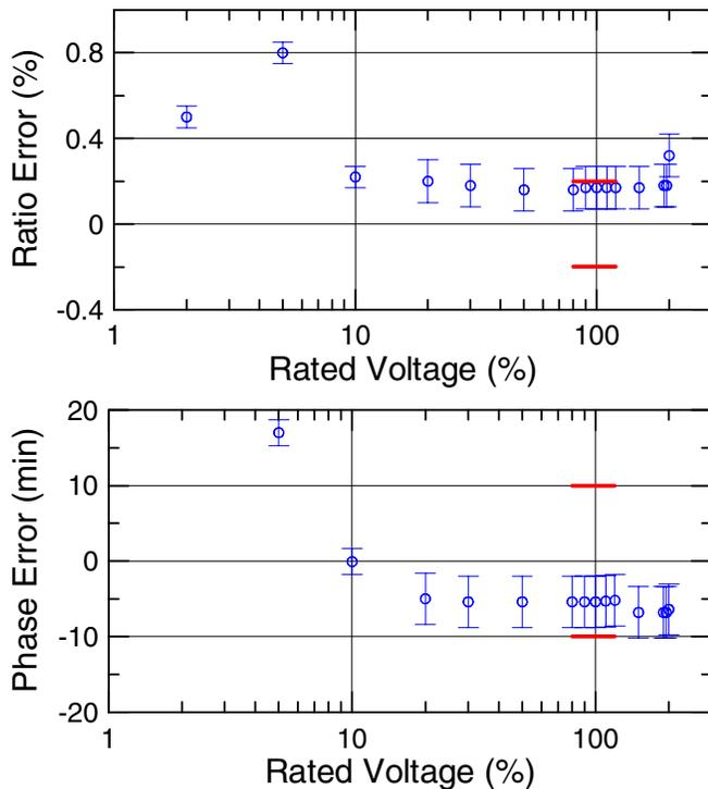
Figure 6. The ratio and phase error of an NXVT LEA output measured at the NRC-Canada. The bars in each graph are the IEC 0.2 accuracy class specification.
