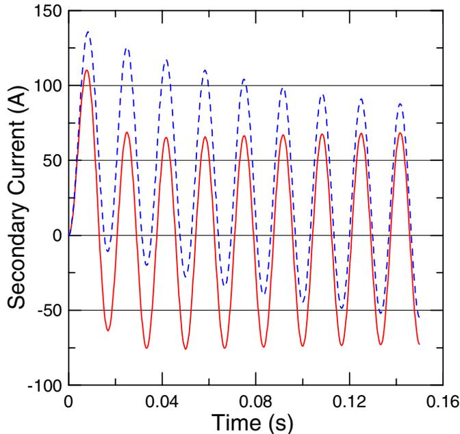
Figure 8. The HEA secondary current from 5 A protection amplifier showing the DC filtered (solid) [IEC TPZ] class and non-filtered output (dashed) [IEC TPE class].
