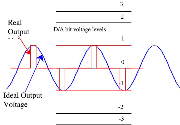
Figure 4. Non-uniform gain and loss of data for a small signal is shown.
