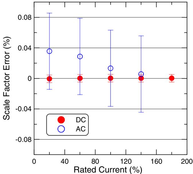
Figure 3. A comparison of the AC and DC measurement capability of a digital NXCT is shown.
