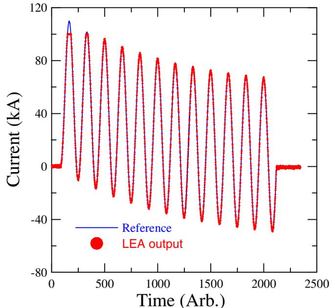
Figure 5. LEA output comparison of a >108 kA peak fully-offset-fault current, (60 Hz frequency).
