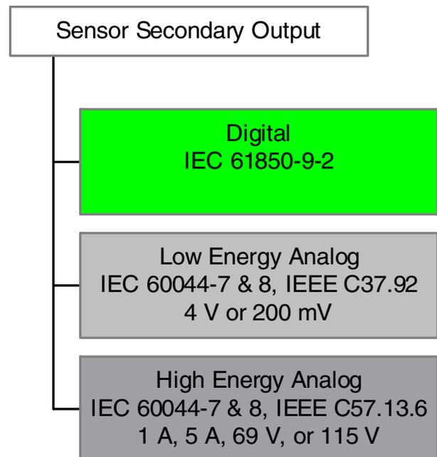
Figure 1. The output categories that a sensor can have according to IEC and IEEE standards.
