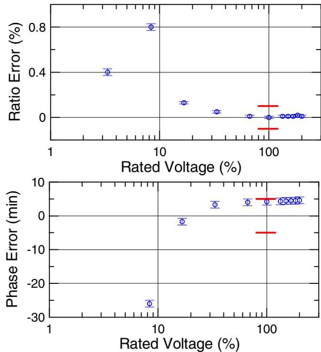
Figure 7. The ratio and phase error for a NXVT HEA output measured at the NRC-Canada. The bars represent the IEC 0.1 accuracy class specification.
