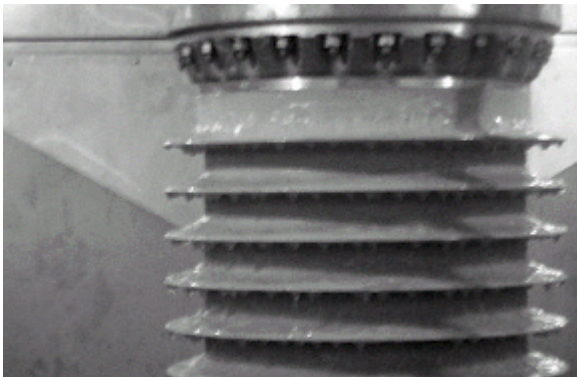
Fig. 5. OVT at the end of the ice test. Chamber temperature ~ 15°C.
