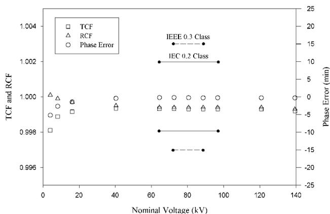
Fig. 2. TCFs, RCFs, and phase errors for the 138 kV OVT.
