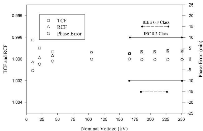
Fig. 3. TCFs, RCFs, and phase errors for the 345 kV OVT.
