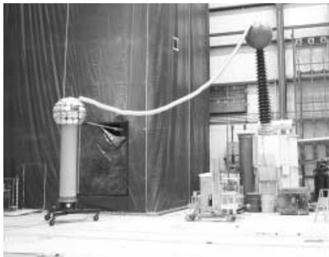
Fig. 1. High-voltage test set-up for fog-pollution tests with reference divider on the left, power transformer (voltage source) on the right, and fog chamber behind them.
