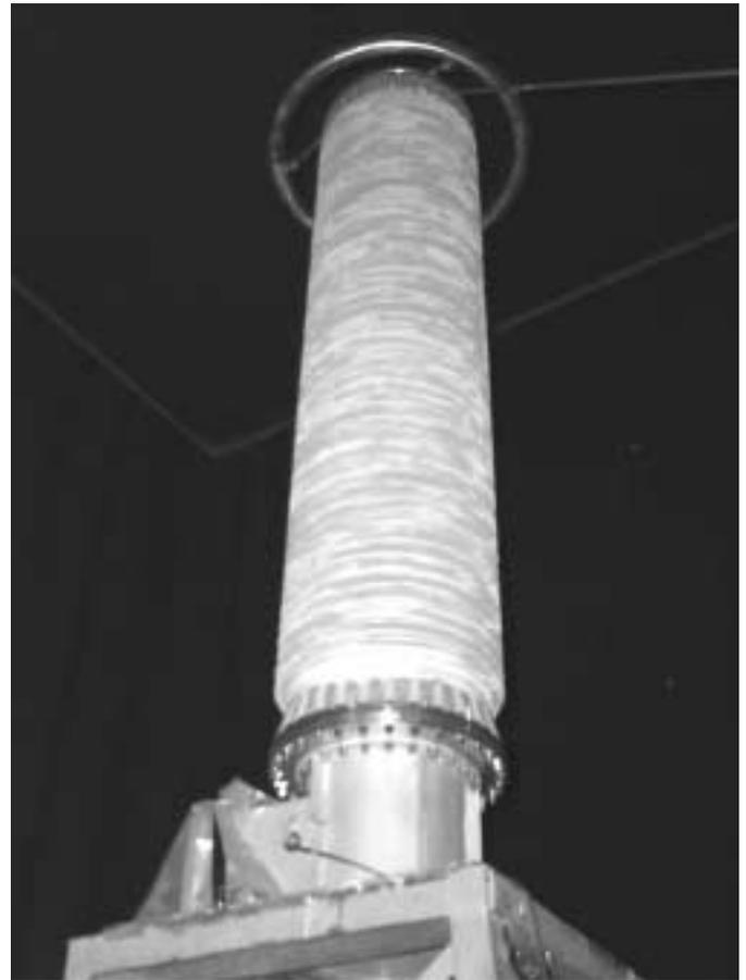
Fig. 2. 345 kV OVT with dried artificial pollution on shed surface.
