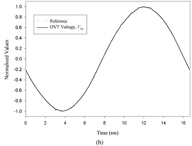
Fig. 3. 345 kV OVT (a) electric fields and (b) voltage waveforms during fog-pollution test.
